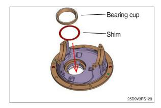
(4) Turn carrier case a on-eighty (180°) and press bearing cup.
