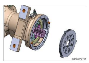
(8) Spread loctite #5127 on axle housing and assemble carrier hsg. sub assembly.
