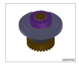
(2) Remove the snap rings, bearings, spacer, and parking gear.
