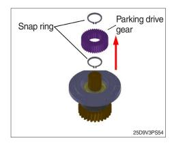
(3) Remove the snap rings, bearings, spacer, parking gear from the parking BRG case.
