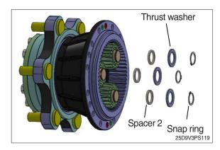
(16) Disassemble planetary gear, needle roller bearing (58EA  $\times$  3= 174EA), spacer 1.
