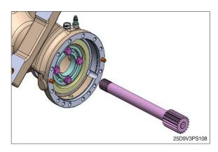
(5) Disassemble special bolt, return spring.
