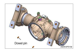
(2) Spread loctite #5127 on axle housing and assemble carrier sub assembly. Spread loctite #277 on the bolt and assemble bolt.
