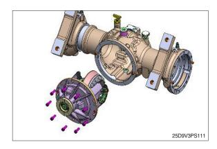
(8) Disassemble Bolt, lock plate.
