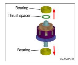
(12) Remove the clutch gear, needle bearing, and thrust washer.
