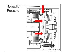
③ Parking brake forced release If no parking release pressure is formed due to engine failure or other causes, vehicle can be moved after forced release of the parking brake.
