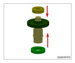
(2) Assembly the piston ring in the groove of the shaft.
