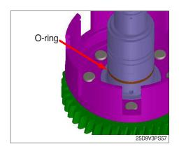
(3) Assemble the piston sub assembly.
