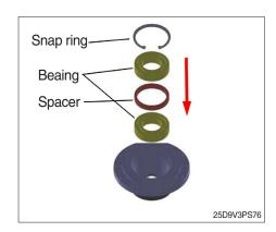
(2) Assemble the parking gear and snap ring.
