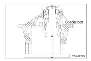
(7) Assemble pinion shaft on spacer.
