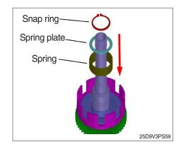
(5) After assembling the plate, disc and pressure plate, the retaining ring is assembled.
