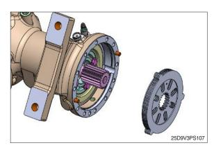
(4) Disassemble axle shaft.
