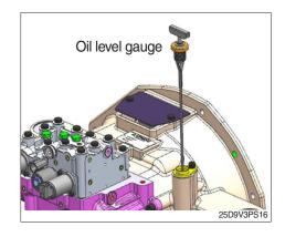
(24) Before putting the transmission into operation, fill it with oil according to operator's manual.
