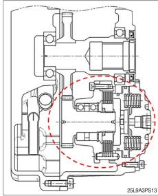
① Parking brake operation The parking spring pushes the piston to squeeze the plate, causing parking brake force by friction force.
