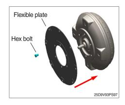
(20) Assemble the torque converter.
