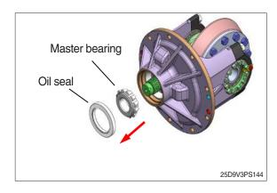
(8) Assemble original taper roller bearing & oil seal.
