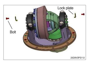
(9) Disassemble bolt, plain washer.
