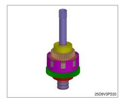
(2) Remove the piston ring and peek seals.
