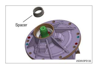
(8) Assemble pinion shaft, and assemble shim & master bearing sort of shim: 0.1, 0.15, 0.3 mm
