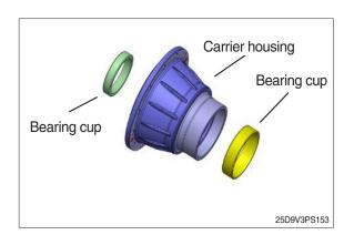
(4) Press T/R bearing and P.L carrier sub assembly.
