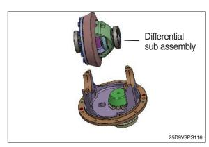
(13) Dissassemble carrier cap, steel ball.
