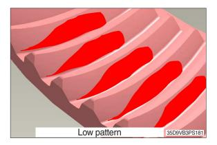
\*\* The good contact pattern of used gearset is appeared what the length of tooth has had as wear pattern.
