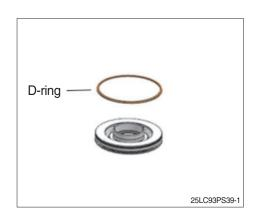
(9) Disassemble the reverse clutch.
