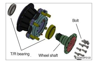
(19) Disassemble hub sub assembly, carrier housing.
