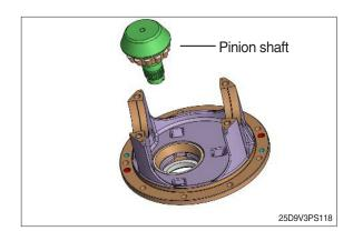
(15) Disassemble Pinion shaft.
