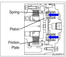
② Parking brake release Hydraulic pressure is applied to the piston from the TM control valve as the piston compresses the spring, the plate is released.
