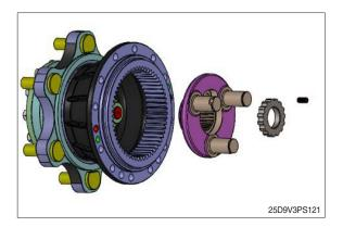
(18) Disassemble bolt, wheel shaft and T/R bearing.
