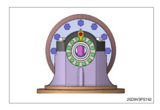
(6) Disassemble lock nut & O-ring & flange yoke.
