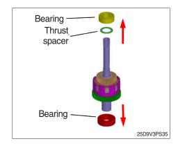
(4) Remove the clutch gear, needle bearing, and thrust washer.
