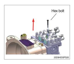
② Remove the control valve and gasket.
