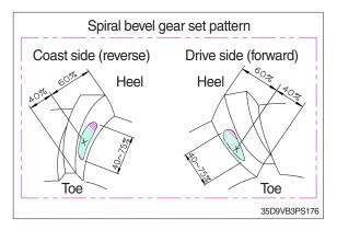
Always check tooth contact pattern on the driving side of gear teeth.
