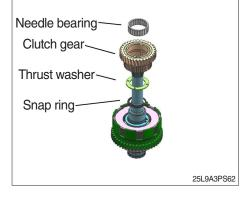
(8) Assemble the thrust spacer and bearing.
