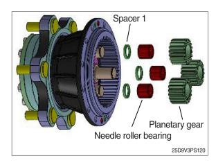
(17) Disassemble set screw, hub lock nut and PL carrier
