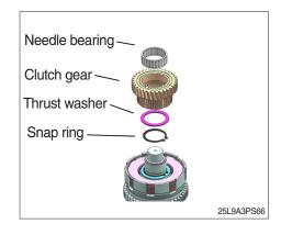
(12) Assemble the thrust spacer and bearing.
