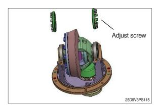
(12) Disassemble differential sub assembly.
