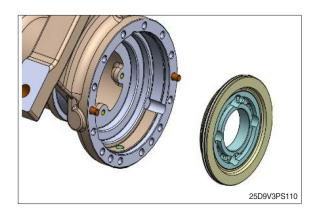
(7) Disassemble bolt, carrier sub assembly.
