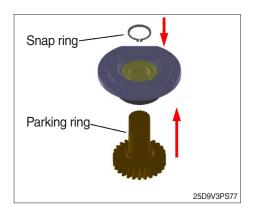
(3) Assemble the snap rings and the parking drive gear.
